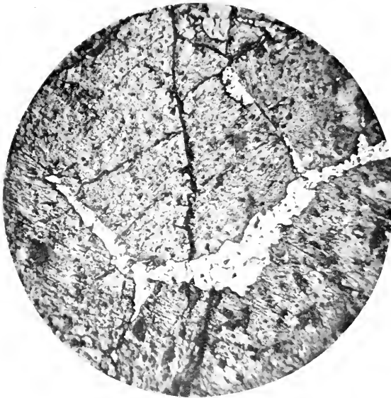
Polished and etched surface of ore, showing pentlandite in veins cutting pyrrhotite; magnified 50 diameters; Copper Cliff mine, Sudbury area, Ontario.
